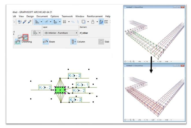
If you want to change all the crownings in the model, select only the crowning components on the Floor Plan. Click on the **"Floating palette / Crowning / Edit Crowning**" command. The solution opens a dialog that shows the available crowning composites on the model. You have to select the number of the crowning structure, which you want to refresh. Click "OK" and the solution will update all the crowning objects (structures) on the Floor Plan that
