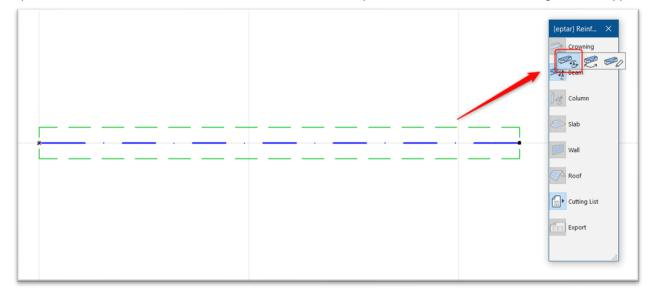
The **rf\_beam** element will be preselected, and you can set all parameters for the current column. These setting are already well known, because the **rf\_beam** element is the same as it was in previous versions. Set all necessary parameters, and click on OK, the addon will place the correct reinforcement in the column construction.
