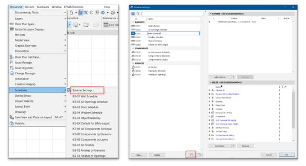
Choose the **"Import...**" button on the right side. Find the installed Reinforcement Library on your computer and the **"[eptar]-Reinforcement.xml**" file in the same location. In most of the cases you can find this file here: **"C:/Program Files/Graphisoft/ArchiCAD/addons/[eptar]\_Reinforcement**".
